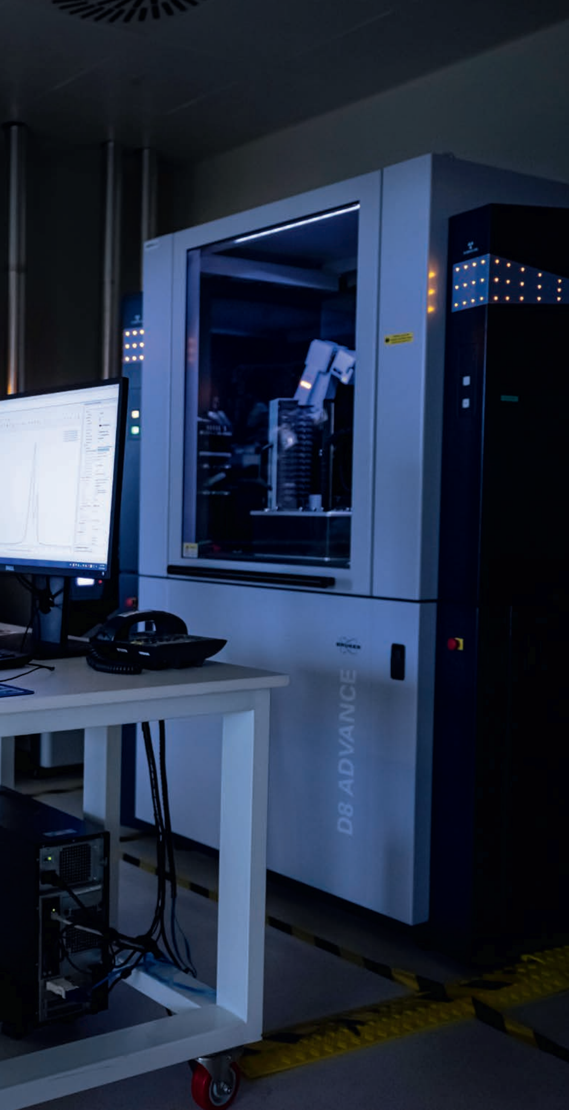
Olivia Zhu, a drug development scientist in China, uses X-ray powder diffraction to study the crystal form of a drug.
